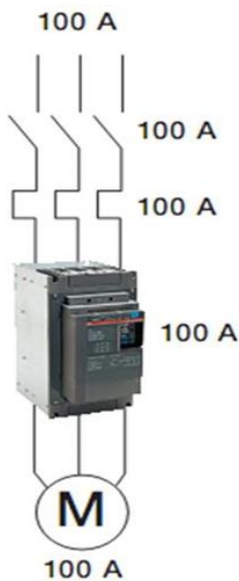
Softstarter connected In-line with the motor
